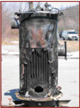
The safety of hot water heaters depends on their maintenance and regular inspections. When a hot water heater is not well-maintained, the potential for damage is explosive.
